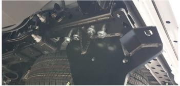
secure with 4x M12x1.25x 40 Bolts with flat washers & nuts.
