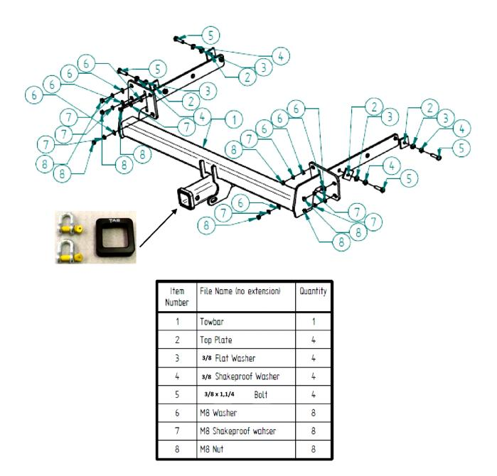
Tools Required: Spanners, Screwdriver, Sockets, Torque wrench
