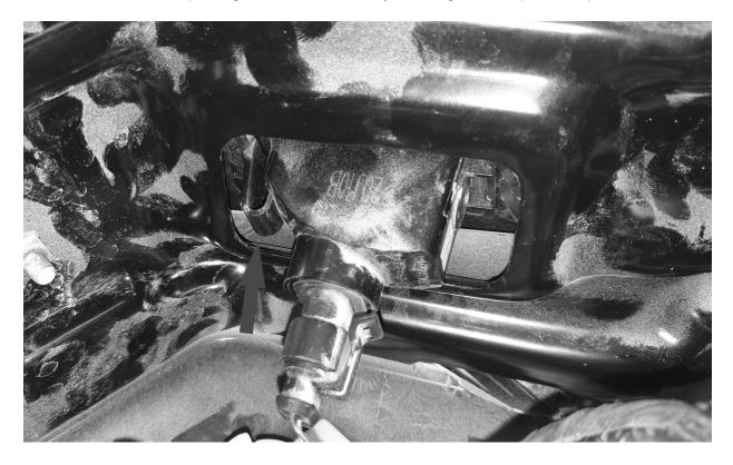
d. Remove 6x 10mm head bolts from the underside of the bumper & 2x 10mm head bolts from the number plate area.
