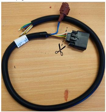
f. Splice the corresponding coloured wires into the vehicle harness. It is recommended to splice and solder the wires however, Scotch Locks may be used.
