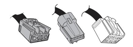
k. Plug in the included Trailer CAN Bus Harness to the 3 corresponding plugs and plug in the Trailer CAN module to its corresponding plug.
