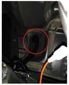
o. Route the tail harness toward the plug mount of the towbar and connect the 7-pin flat plug as per the diagram (pg2).
