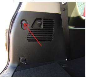
h. Remove the lower tie-down fixture by lifting plastic flap and removing its securing bolt. Repeat on opposite side.
