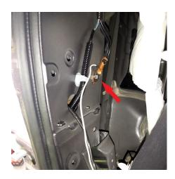
n. On LHS, locate the large round grommet at the lowest point behind the trim. Make a small incision and feed the tail harness (7 core) through to the outside.
