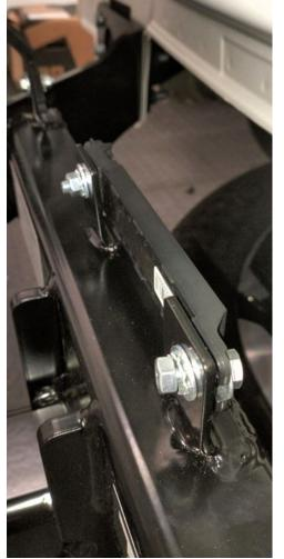
**MQ4 PE 11/2023-on** Plastic Bumper mounts. Take note of orientation when removing them from the crash bar.
