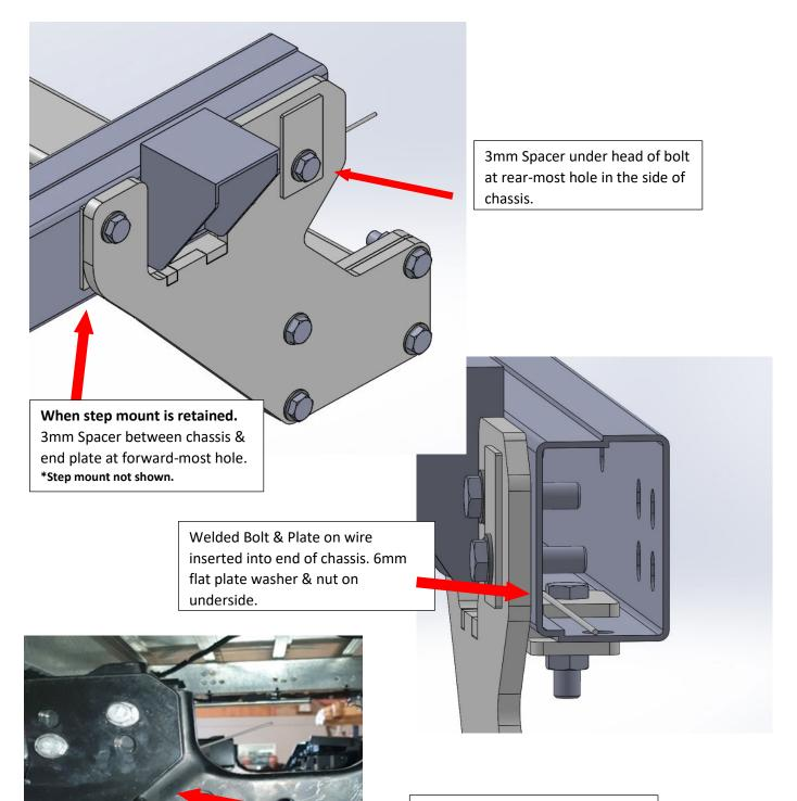
Step mount is retained between chassis & end plate.
