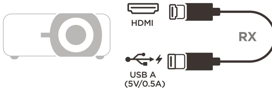
1. Connect the Receiver's HDMI Output to an **HDMI** port of the projector.
