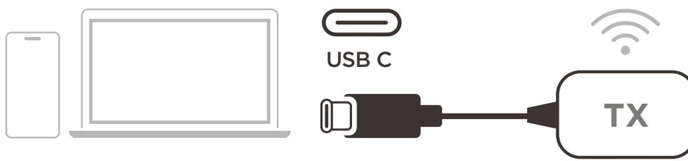
1. Connect the Transmitter's USB C Input to a **USB C** port of the casting device (e.g. laptop, mobile phone, tablet).
