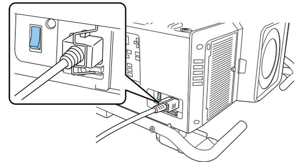
The projector's power indicator turns blue (it is in standby mode). This indicates that the projector is receiving power, but is not yet turned on.
