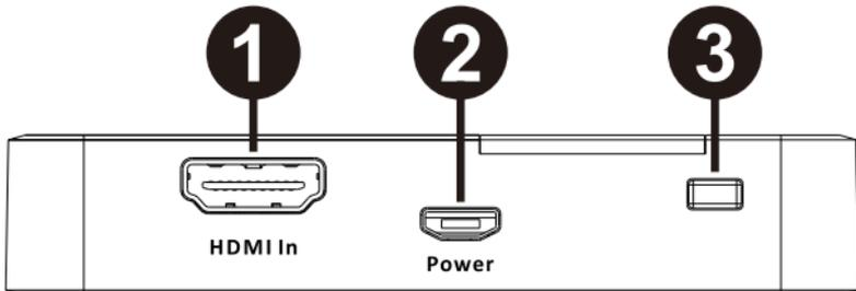
1. **HDMI IN:** This slot is where you connect the HDMI source.
