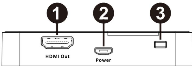
1. **HDMI OUT:** This slot is where you connect to a HDMI equipped TV or monitor.
