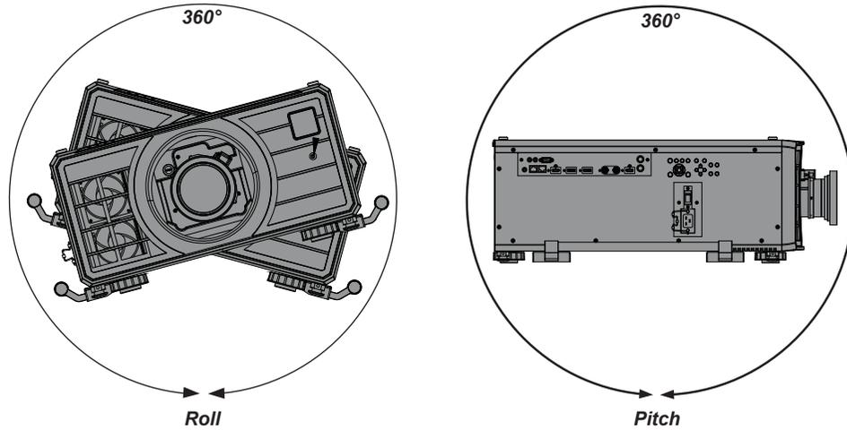
**Fig. 1 Roll and pitch - any position is possible**
