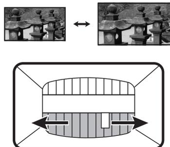
To improve the clarity of the image, rotate the Focus Ring.
