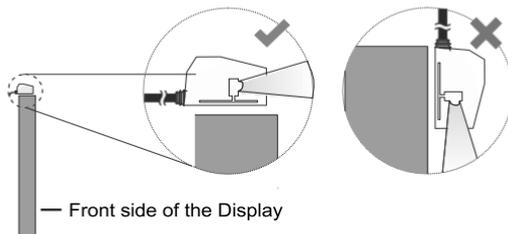
Depending on the model, your Display may have a built-in IR receiver on its cabinet. This IR receiver will not function if the external IR receiver is connected to the Display. Disconnect the external IR receiver if you want to use the built-in IR receiver again.
