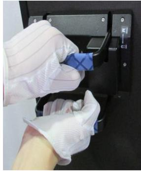
Step 5. Ensure the magnet is locked. Detach the tile carefully.
