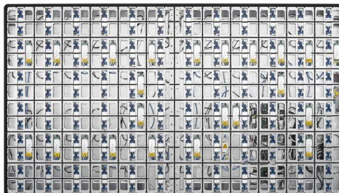
**Step 2.** Loosening 3pcs black M3 flat head screws from both upper and lower sides of panel.
