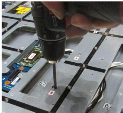
**Step 5.** Install and tighten 3 pcs black M4 flat head screws to both upper and lower side of the case.
