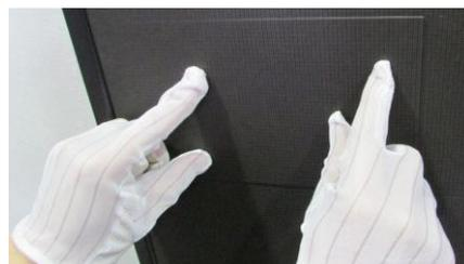
**Note: When mounting an intelligent module back, pay more attention to the guide pin which is located in corners to mount it smoothly.**
