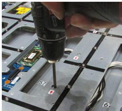
**Step 8.** Holding the reinforced rib and disassemble the display.
