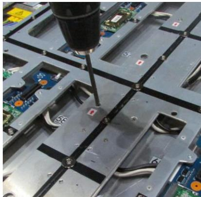
**Step4.** Install 11 pcs M4 button head cap screws(with a plain washer and spring washer).
