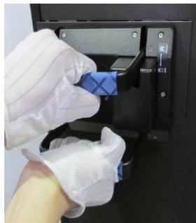
Step 6. Put down the intelligent module and tool together carefully onto an EPE (or other soft pad).
