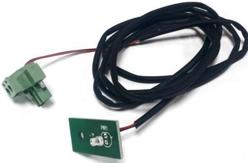
Figure 3 Ambient Light Sensor
