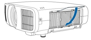
Close the air filter cover and tighten the screws.
