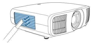
**3** Loosen the screws and remove the air filter cover.
