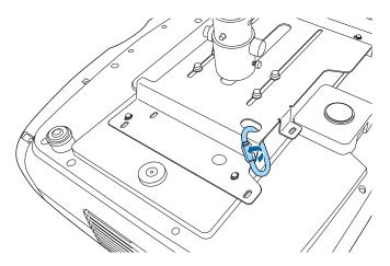
Attach the wire clamp to another carabiner, and then use the screw to fix the wire clamp to the wire clamp fixing point on the projector.
