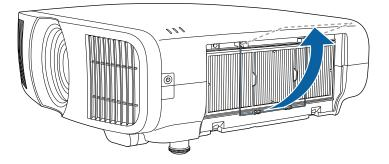
Pull the air filter out of the projector.
