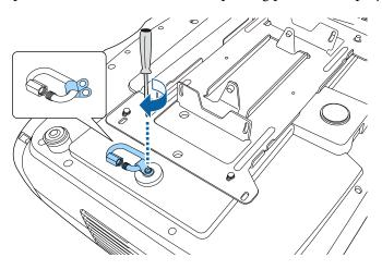
2 Loop the safety wire through the hole in the ceiling mount, and then attach both ends to the carabiner.
