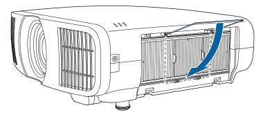
10 Close the air filter cover and tighten the screws.
