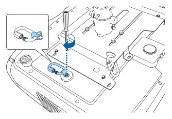
Loop the safety wire through the carabiner on the ceiling mount, and attach both ends to the carabiner on the projector.
