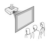
Select the correct **Projection** option in the projector's **Installation** menu according to the installation method being used. If necessary, turn on the **Inv Direction Button** setting in the projector's **Operation** menu.
