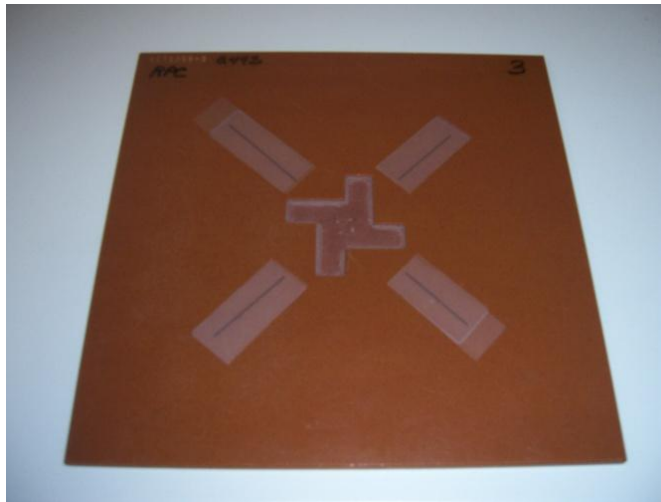
Figure 2.7 Solid Water phantom.
