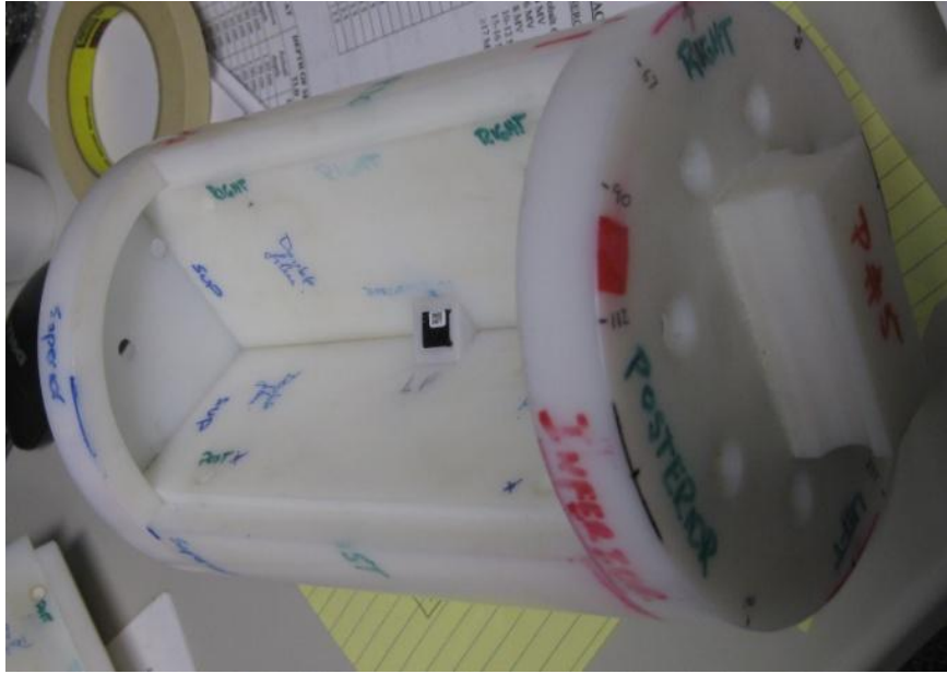
Figure 2.9 HIPS dosimetry insert with section removed showing one OSLD.
