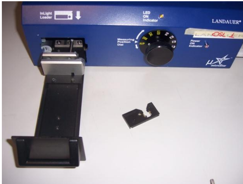
Figure 2.3 MicroStar reader with drawer extended showing the OSLD insert area.
