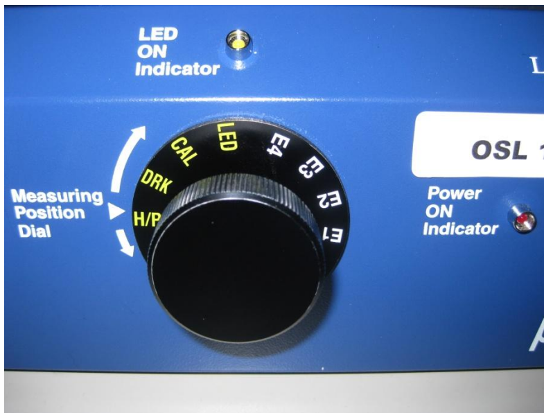
Figure 2.4 MicroStar knob control allowing selection of QA measurements or dosimeter readout.
