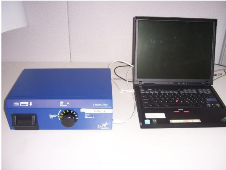
Figure 2.2 MicroStar reader with accompanying computer with microStar software.
