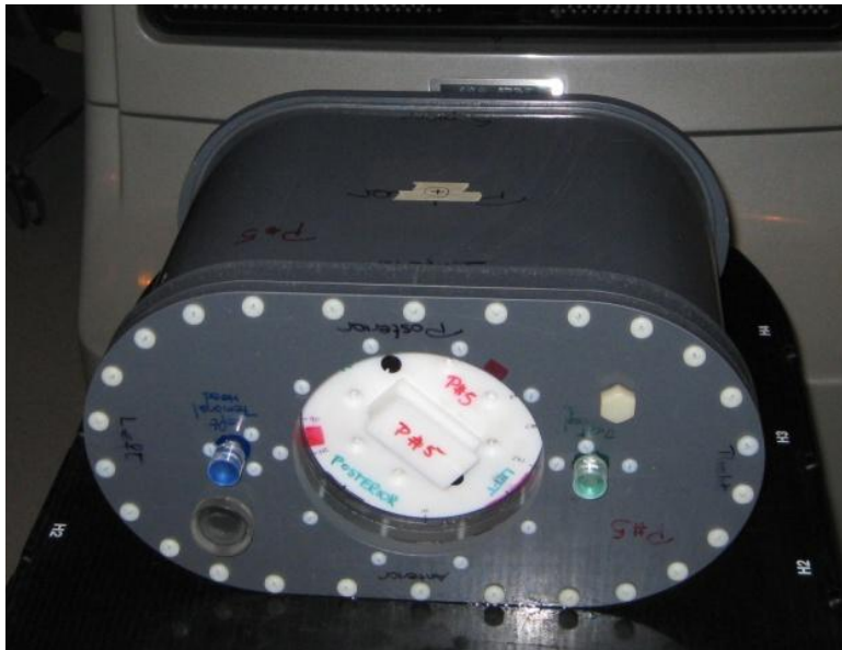
Figure 2.8 Pelvic phantom front view.
