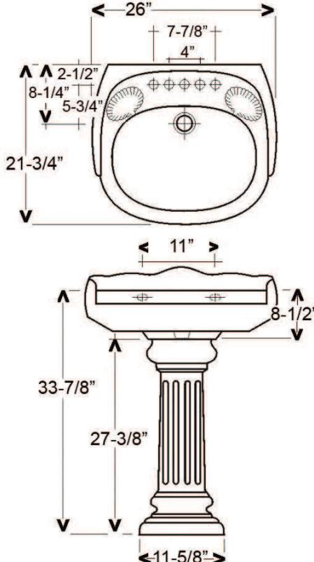
Dimensions of fixture are nominal and may vary within the range of tolerances established by ASME Standard A112.19.2-2008. Dimensions and specifications subject to change without notice.
