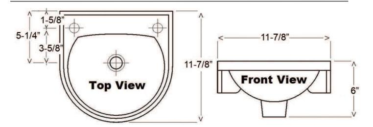
Dimensions of fixture are nominal and may vary within the range of tolerances established by ASME Standard A112.19.2. Dimensions and specifications subject to change without notice.
