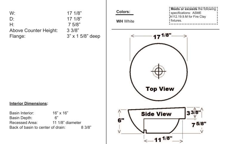
Dimensions of fixture are nominal and may vary within the range of tolerances established by ASME Standard A112.19.2. Dimensions and specifications subject to change without notice.
