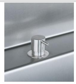
Stop valve with ¼ turn ceramic disc technology. Includes non-return valve and ½" inlet/outlet. Hole cut out size: 28 mm max 35 mm.
