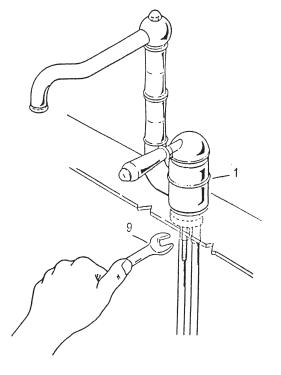
Check the position on the sink of the faucet, then tighten the nut with a 13mm wrench.
