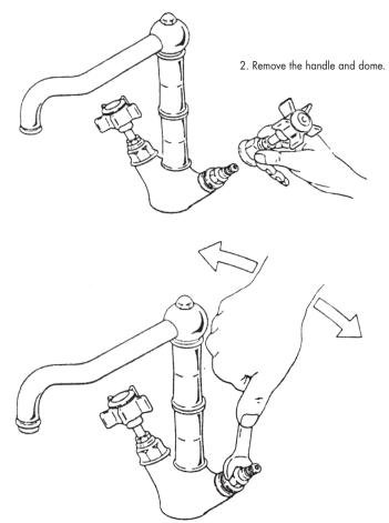
3. Remove the cartridge with a smooth jawed wrench or 17mm wrench
