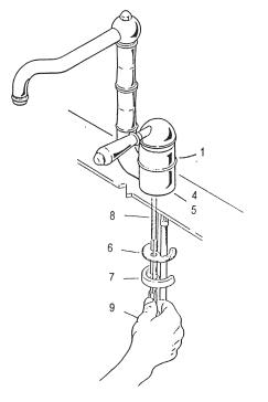
Under the sink, stack the half ring rubber gasket - 6, the half ring mouting plate - 7, then the mounting nut -9 onto the stud.
