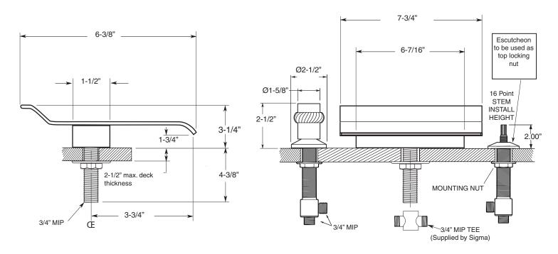
NOTE: Spout and valves install through 1-1/4" diameter holes.
