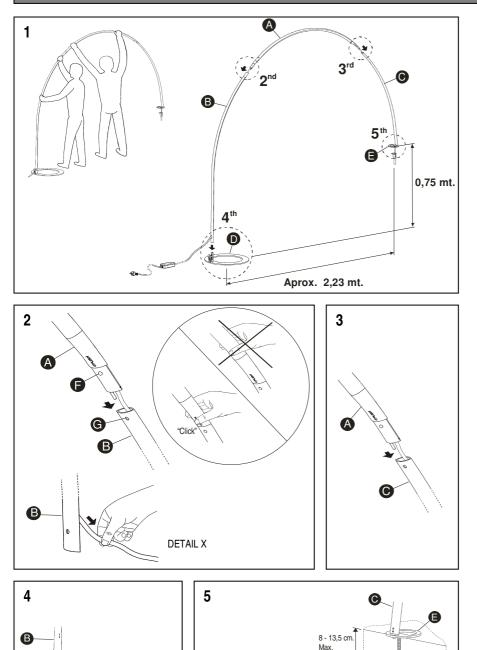
**1.** Remove the top (A) and side (B and C) profiles from the carry bag and lay them out. Place the base (D) where you want to install the lamp. Keep in mind that the distance between the center of the base and the fixation point must be 2.23 mt. Approx.
