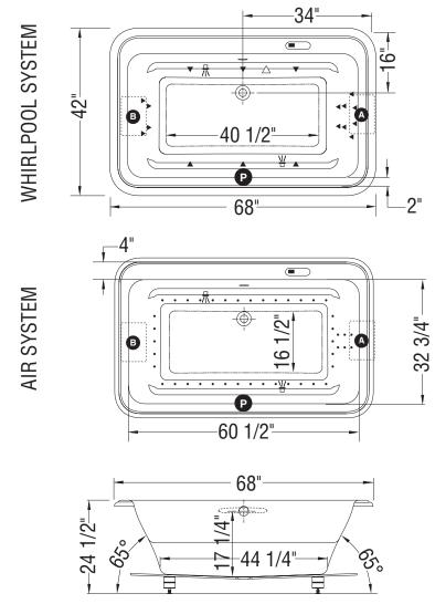
Note: The backjets are always on opposite side of blower or pump. In combined system, the backrest is on same side as remote blower.
