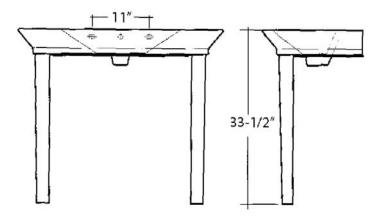
Dimensions of fixture are nominal and may vary within the range of tolerances established by ASME Standard A112.19.2. Dimensions and specifications subject to change without notice.
