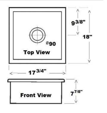
Dimensions of fixture are nominal and may vary within the range of tolerances established by ANSI Standard A112.19.9. Dimensions and specifications subject to change without notice.
