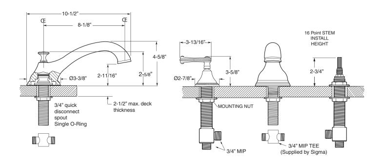
NOTE: Spout and valves install through 1-1/4" diameter holes.
