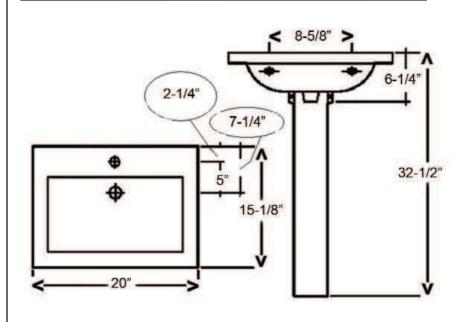
Dimensions of fixture are nominal and may vary within the range of tolerances established by ASME Standard A112.19.2-2008. Dimensions and specifications subject to change without notice.
