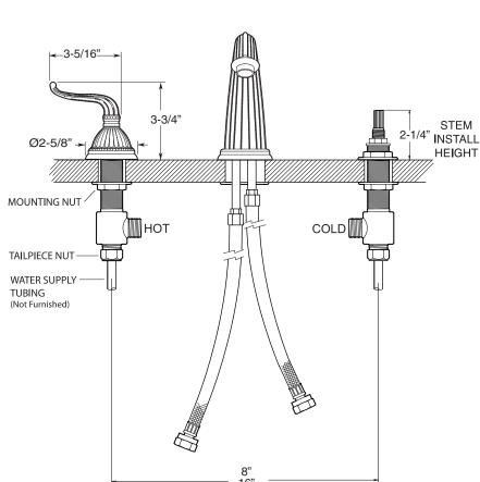
NOTE: Spout and valves install through 1-1/4" diameter holes
