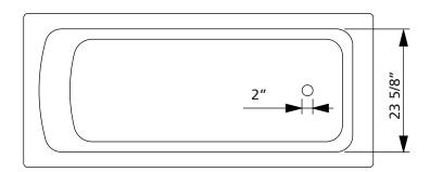
Note: Adjustable feet raise tub 3 1/4" to 6 1/4" from floor to bottom of drain hole.
