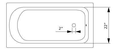
Note: Adjustable feet raise tub 3 1/4" to 6 1/4" from floor to bottom of drain hole.
