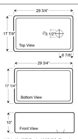
Dimensions of fixture are nominal and may vary within the range of tolerances established by ANSI Standard A112.19.2. Dimensions and specifications subject to change without notice.
