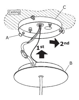
**5-** Reinstall the base (B) as shown by the arrows. Tighten the screws (A) to fix the lamp to the plaque (C).
