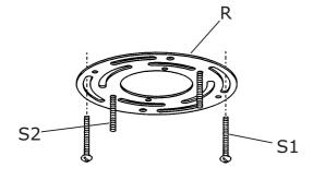
**1-** Making certain that the threads of the cross bar screws are pointing away from the ceilingl, secure the round cross bar (R) to the junction box using the mounting screws (S1) after inserting the screws (S2) from within out.
