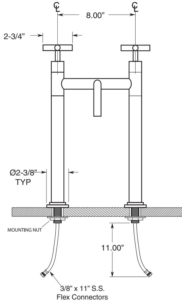
NOTE: Install through 1-1/4" diameter holes
