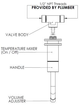
4. Tighten the mixer to the valve body with the allen set screw
