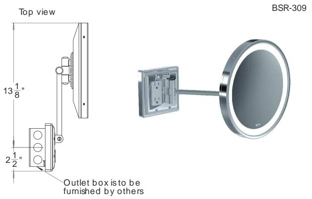
The center of the mirror is 7/8 " above the center of the outlet box. Since the typical user's eye height is 58 3/4" the outlet box should be centered 57 7/8" above the floor
