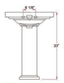
Dimensions of fixture are nominal and may vary within the range of tolerances established by ASME Standard A112.19.2-2008. Dimensions and specifications subject to change without notice.
