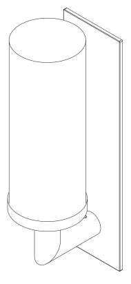
\* Installation Note (Electrician/Wall-finisher): This light uses a non-standard size backplate. This light is designed to be installed onto a standard vertically installed switch box. Maximum width of finished opening is 2-1/2".
