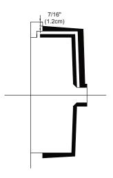
By IAPMO, ceramic lavatory warpage is defective only if warpage of flat slab out of horizontal plane exceeds 6.3 mm/m (0.25 in/ft) on all sizes OR warpage on back of lavatories that are attached to the wall exceeds 3 mm (0.13 in).
