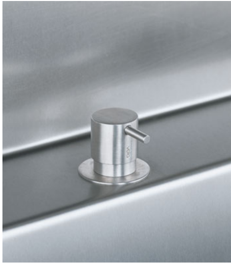
S50 Stop valve with ¼ turn ceramic disc technology. Includes non-return valve and ½" inlet/outlet. Hole cut out size: 28 mm max 35 mm.
