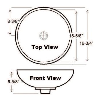
Dimensions of fixture are nominal and may vary within the range of tolerances established by AMSE Standard A112.19.9. Dimensions and specifications subject to change without notice.
