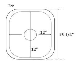
Dimensions of fixture are nominal and may vary within the range of tolerances established by ANSI Standard A112.19.2. Dimensions and specifications subject to change without notice.
