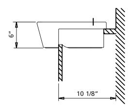
Note: Must have minimum 10 1/8" from wall to groove.
