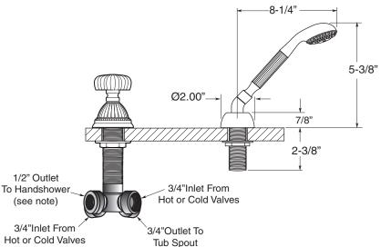
Spout and valves install through 1-1/4" diameter holes.
