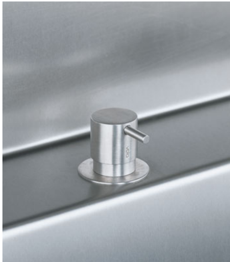
S50 Stop valve with 1/4 turn ceramic disc technology. Includes non-return valve and 1/2" inlet/outlet. Hole cut out size: 28 mm max 35 mm.
