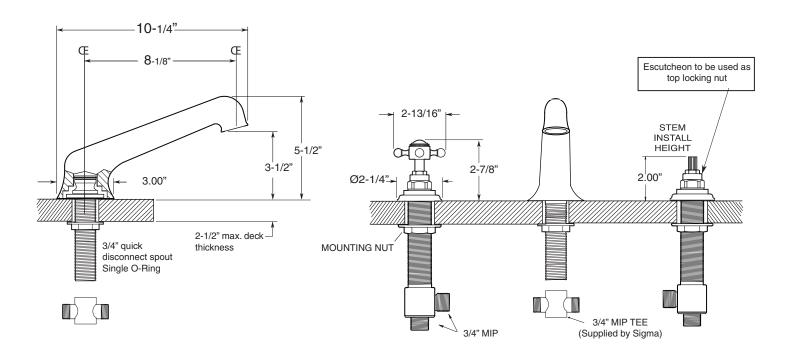
NOTE: Spout and valves install through 1-1/4" diameter holes. Plumber to provide 3/4" supply lines to valves
