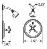
Flow Rate: 5.8GPM@50PSI
