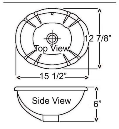
Dimensions of fixture are nominal and may vary within the range of tolerances established by ASME Standard A112.19.2. Dimensions and specifications subject to change without notice.
